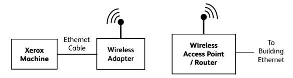
The Wireless Adapter (also known as an Ethernet-to-Wireless bridge) is a device that connects into the machine's Ethernet port using an Ethernet cable and acts as a wireless to wired Ethernet converter.
